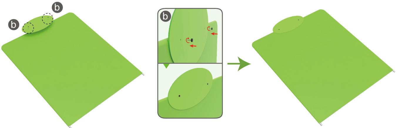
**STEP 02** Insert display stands onto feet by pressing their knobs.
