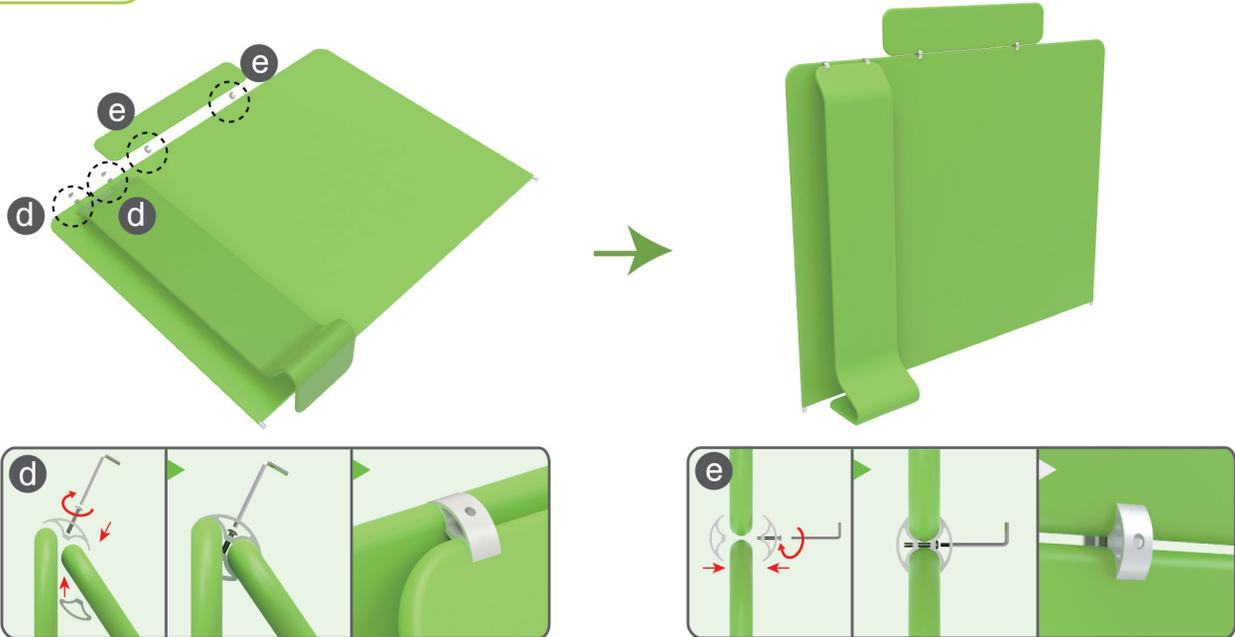
**STEP 02** Insert display stands onto feet by pressing their knobs.
